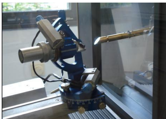
Collimator with mirror which is transparent for x-rays allows the real time imaging of both the Laue Pattern and the optical image simultaneously
