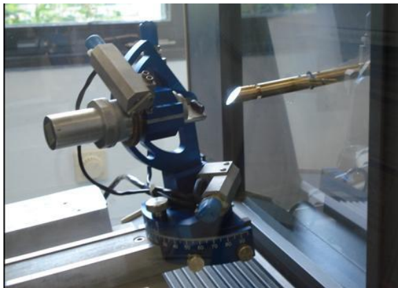
Collimator with mirror which is transparent for x-rays allows the real time imaging of both the Laue Pattern and the optical image simultaneously
