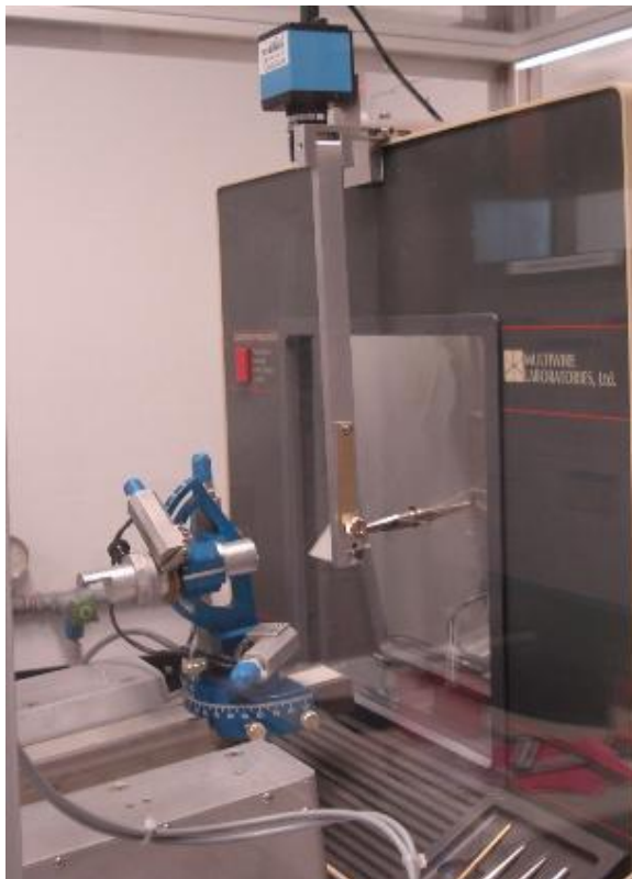
Retractable USB-camera-mirror system for exact positioning of the sample in the beam
