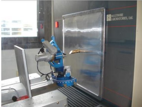
Fluorescence filter and mirror collimator on the MWL 110 detector
